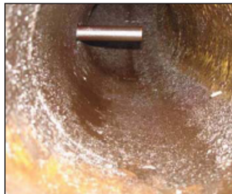
Figures 1, 2: A contaminated lube oil reservoir (left) and system pipeline (right)
