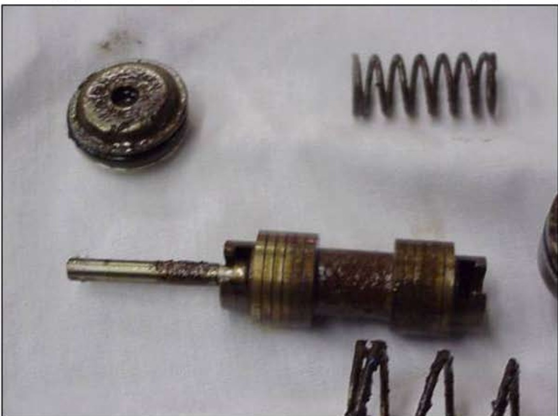
Figure D – VARNISHED VALVE INTERNALS THAT FAILED
