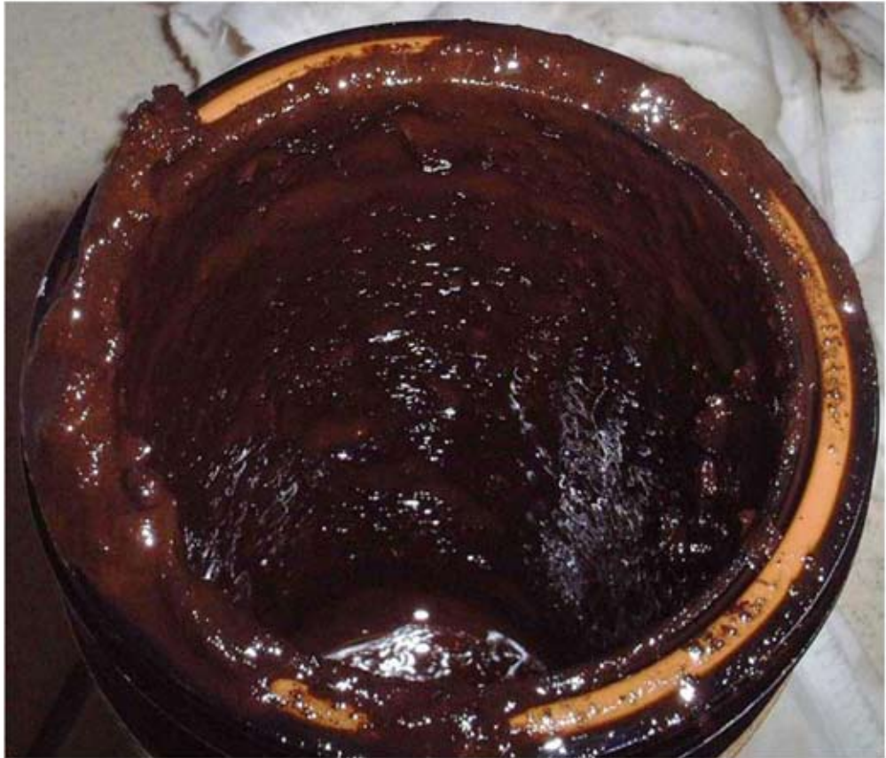
Figure F - TURBINE PIPING INTERNALS SAMPLE - PREVIOUS PROJECT
