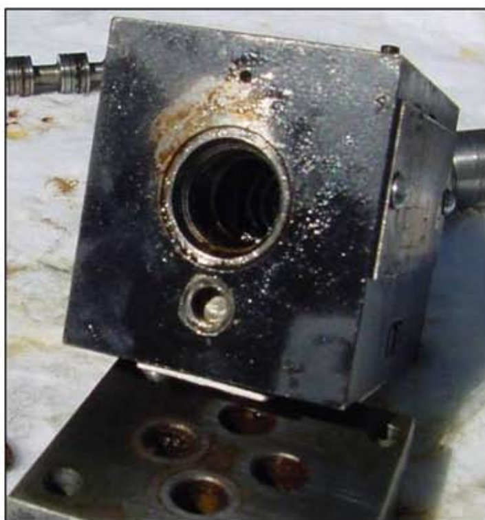
Figure E – VARNISHED VALVE BODY
